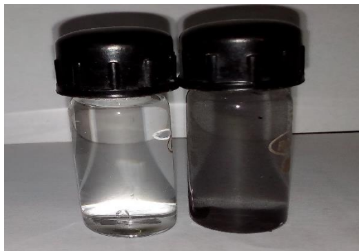
Fig. 1 (a) zinc nitrate solution and (b) color change during the reduction of zinc nitrate into zinc oxide nanoparticle by the extract of Murraya koenigii seeds after 120 hrs of incubation
